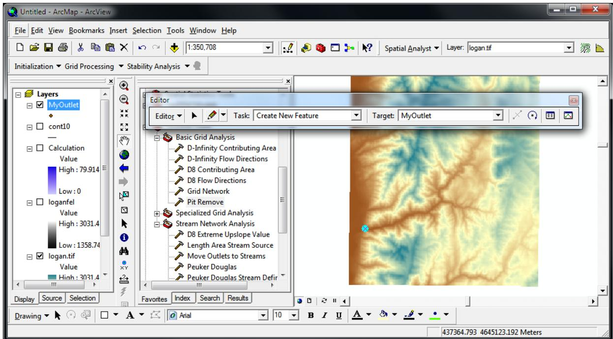
It is not required for the outlet to be precisely located where there will be a stream as TauDEM has a tool to move outlets to streams that will be used. Alternatively, if the outlet point location is available from some other source (e.g. location information about a stream gauge), it can be created from that information.
