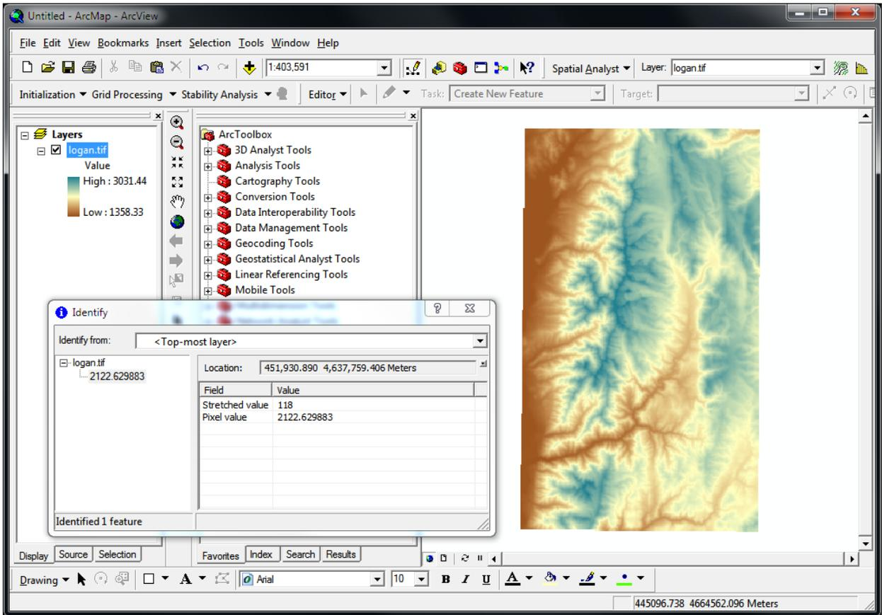
This display also shows the output from clicking on and identifying individual grid values. A DEM grid is a simple data structure that defines elevation values within a matrix of identically-sized square (or in general rectangular) grid cells as illustrated below.
