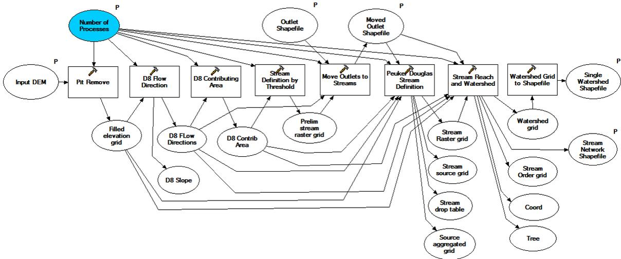
Following through the sequence illustrated in this function you can see the steps involved and how watershed delineation works. The workflow is organized to flow from left to right.
