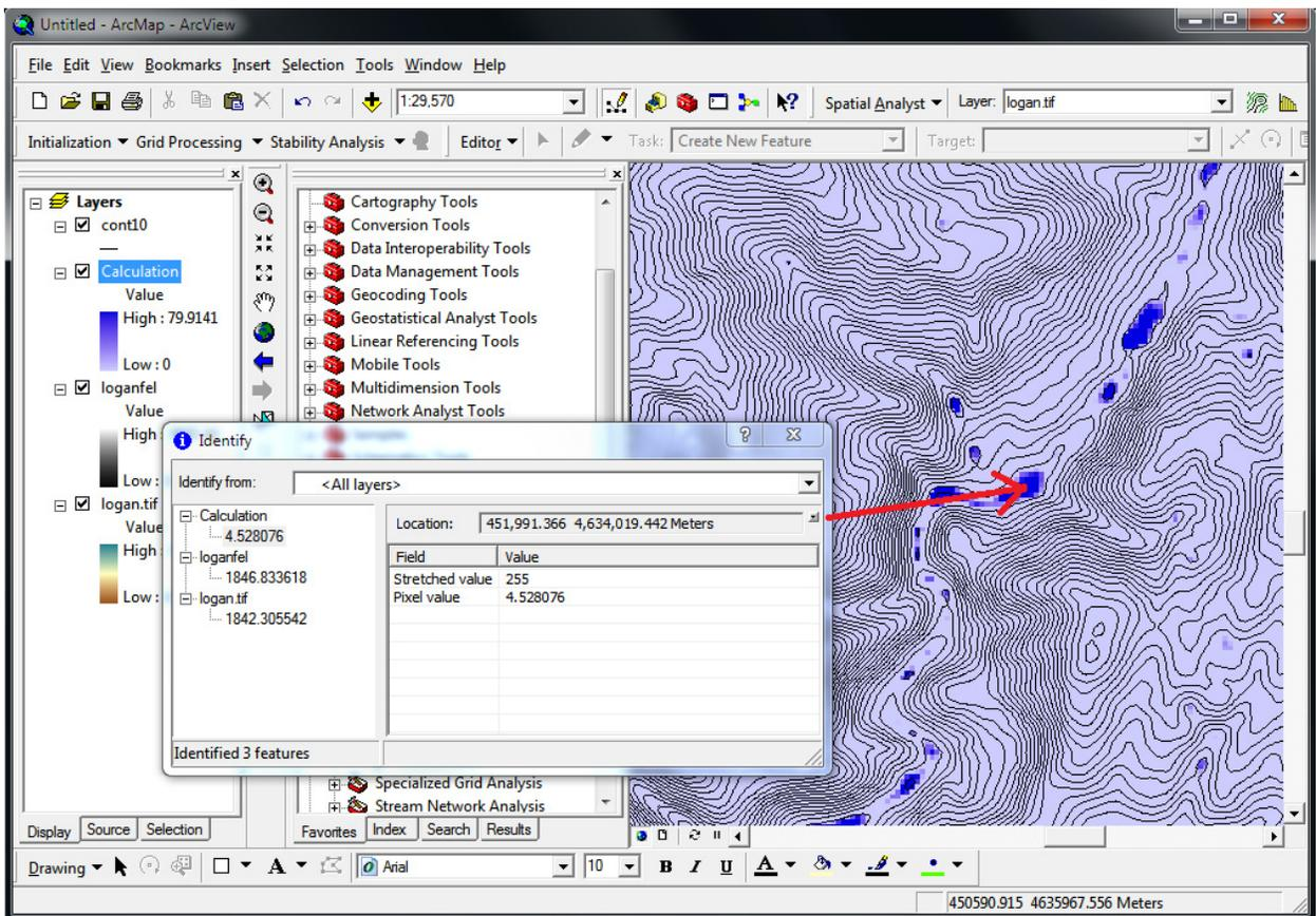
It is common to see pits along valleys where interpolation during the DEM creation process has created artificial barriers (dams) that are resolved by filling. Unless these pits are removed they become sinks
