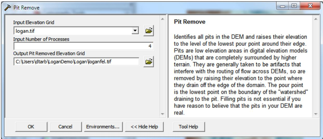
Note how when the Input elevation grid is selected the software automatically fills in output fields using TauDEM's file naming convention. This saves on some of the work involved in running these tools.
