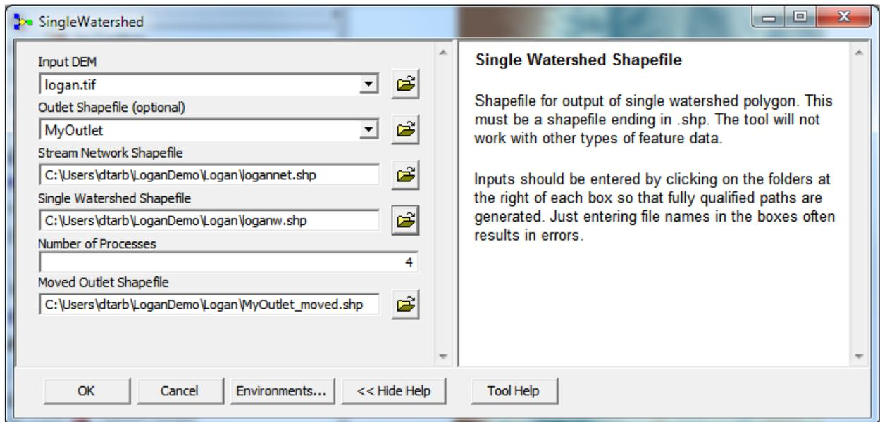
The screen will flash a number of times as each task executes. If all goes well the dialog box should show Completed with no errors and give details of the timing and shell scripts that were executed as part of this process.
