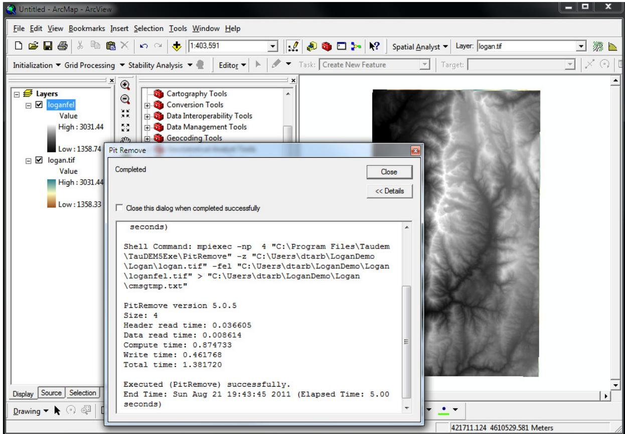
3. Use Spatial Analyst -> Raster calculator to evaluate the difference between the pit filled DEM *loganfel* and original DEM, *logan.tif*. Symbolize the output Calculation and zoom in to analyze some of the differences.
