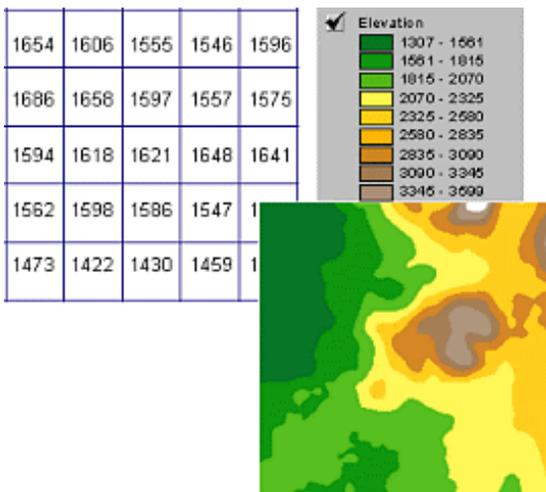
The TauDEM software derives hydrologically useful information from raw digital elevation model data. The basic idea rests on the concept of the hydrological flow field being represented by flow from each
