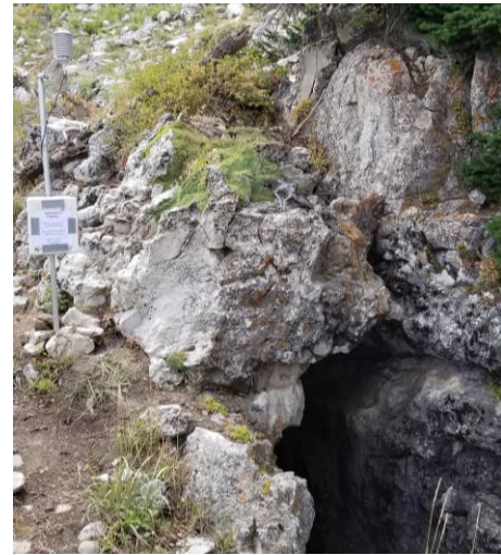
Figure 3: One of the remote stations deployed to identify differences in temp. and RH between karst features and the surrounding areas.
