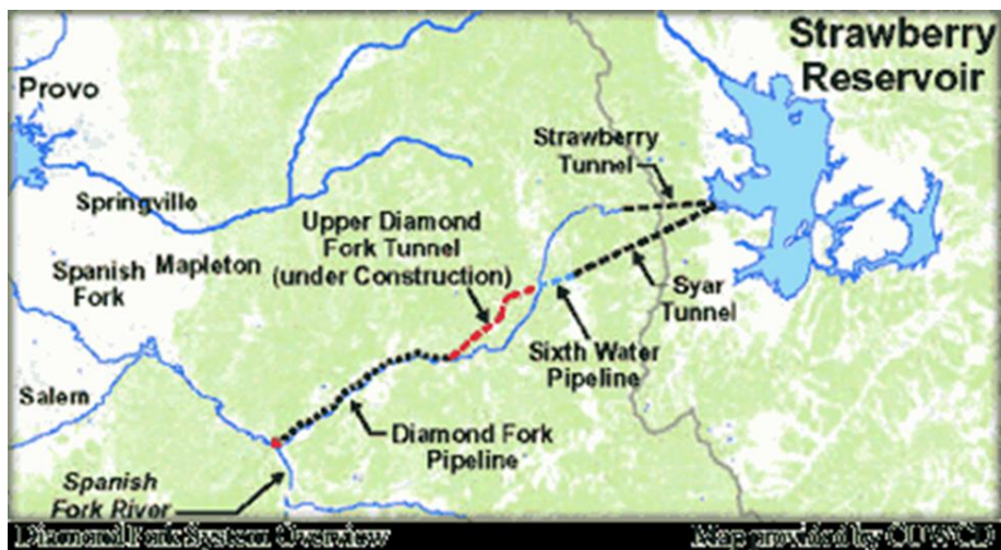
Figure 2. Diamond Fork Irrigation Delivery System.
