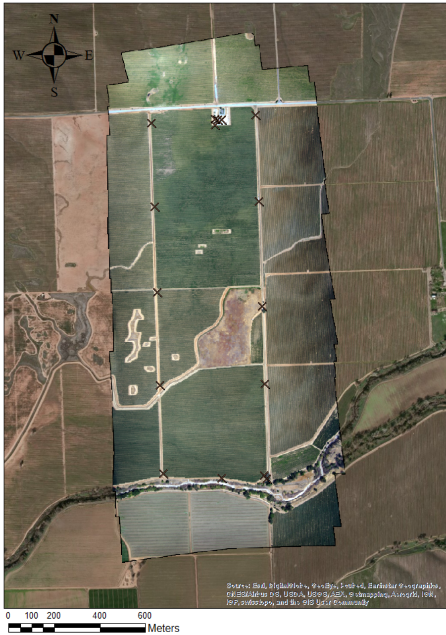
FIGURE 3: RGB MAP GENERATED BY ARCMAP OVER ESRI WORLD IMAGERY BASEMAP. THE X PRESENT ON THE MAP REPRESENT THE LOCATION OF THE CONTROL POINTS.
