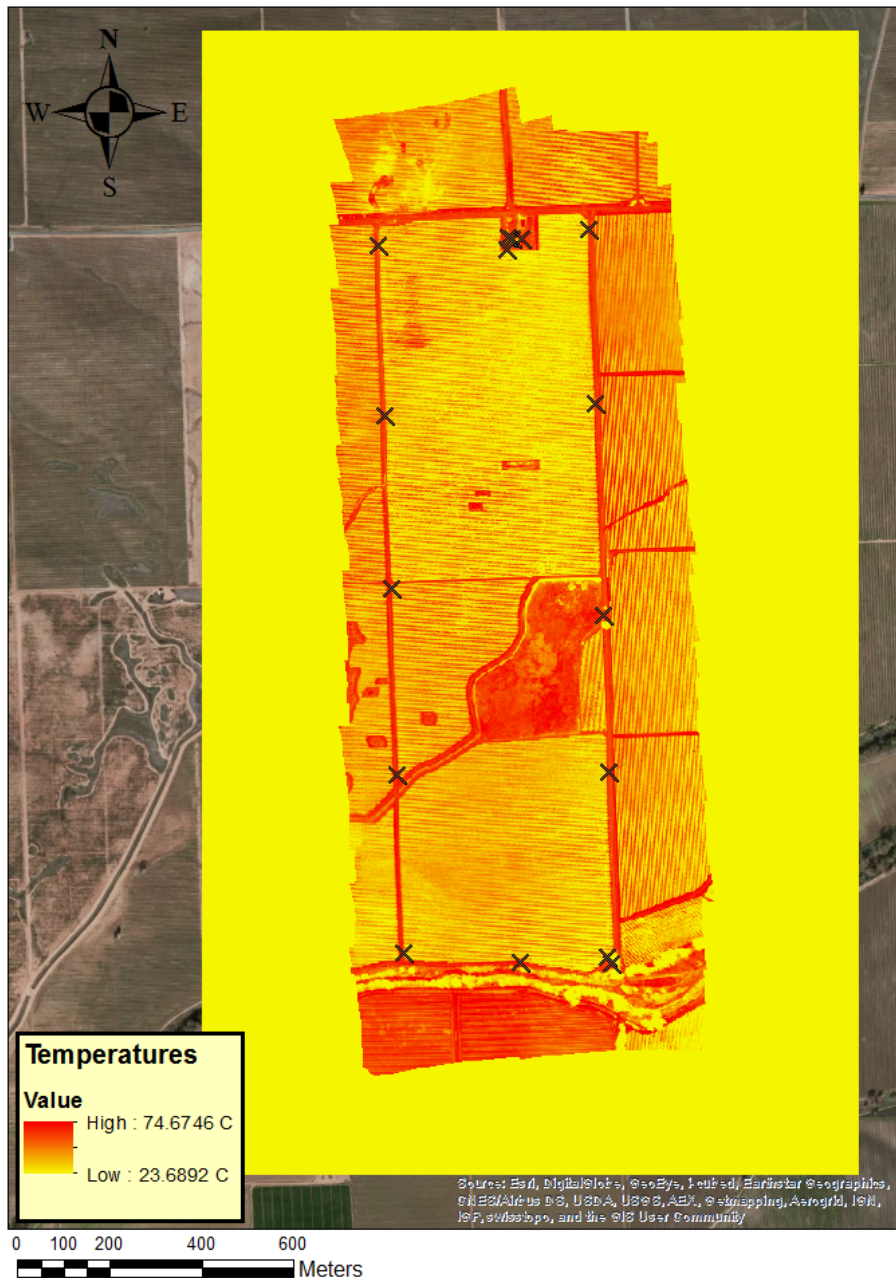
FIGURE 6: THERMAL MAP OF AFTERNOON AGGIEAIR FLIGHT, GENERATED BY ARCMAP OVER ESRI WORLD IMAGERY BASEMAP. THE X PRESENT ON THE MAP REPRESENT THE LOCATION OF THE CONTROL POINTS.
