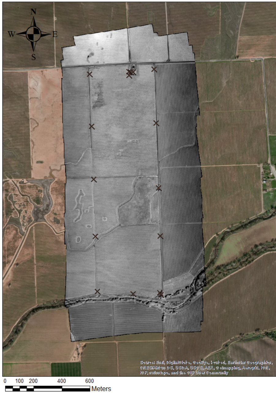
FIGURE 4: NIR MAP GENERATED BY ARCMAP OVER ESRI WORLD IMAGERY BASEMAP. THE X PRESENT ON THE MAP REPRESENT THE LOCATION OF THE CONTROL POINTS.
