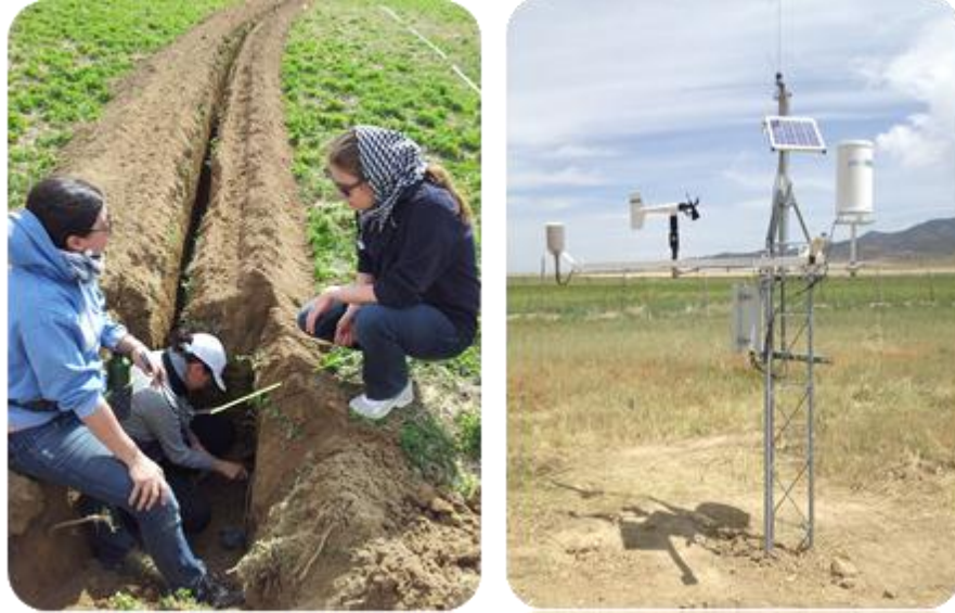
Figure 3 To the left: placing the sensors at one and two foot, to the right the weather station
