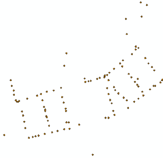
Figure 1 Incorrect Layout of Tuni Grande's Distribution System. Both x and y coordinates should be negative to represent a west and southern location.
