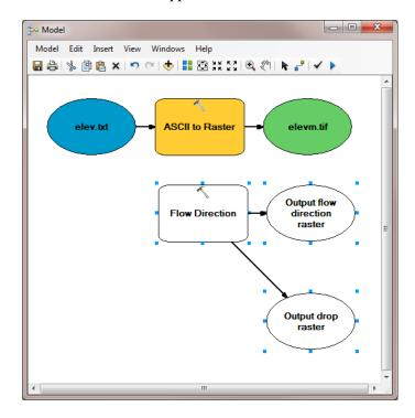
The output from the ASCII to raster function needs to be taken as input to the Flow Direction function. To do this use the connection tool and draw a line from **elevm.tif**, the Output raster of ASCII to Raster, to the Flow Direction tool rectangle. At the dialog that pops up select **Input surface raster** to indicate that elevm.tif is to be used as the input Surface raster for the Flow Direction tool.
