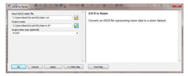
Set the Input ASCII raster file to **elev.txt** and Output raster to **elevm.tif** (I used elevm.tif so as not to conflict with elev.tif that already exists). Set the output data type to be FLOAT. Click OK to dismiss this dialog. Note that the model elements on the ModelBuilder palette are now colored indicating that their inputs are complete.
