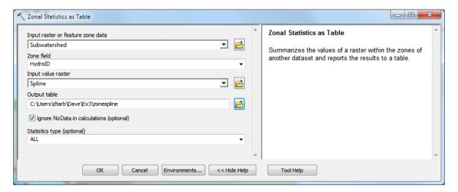
Click OK. A table with zonal statistics is created. This contains statistics of the value raster, in this case mean annual precipitation from **Spline** over the zones defined by the polygon feature class **Subwatershed**. The HydroID in this table may be used to join it to the attribute table for the Subwatershed feature class. As for the elevations above this joined table can be exported and examined and presented in Excel.
