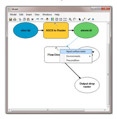
Notice that the "output drop" oval is hollow. This is because this is an optional output that has not been specified. Double click on the Flow Direction tool and specify names for both the Output flow direction raster and optional Output drop raster.
