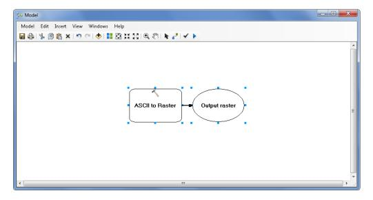
Double click on the **ASCII to Raster rectangle** to set this tool's inputs and outputs.
