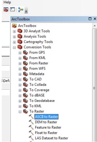
Specify the name of the Output raster as **elev.tif** and give it a disk location. (Note that the extension specifies the grid file format, .tif for a TIFF file, .img for an ERDAS IMAGINE file, or no extension for an ESRI GRID raster format.) Specify the Output data type as **FLOAT** because the given elevation data includes decimal values.
