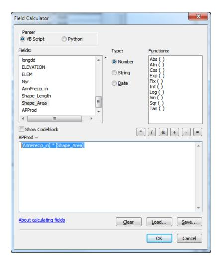
The result is a new field with the numerator terms for the equation above. Now locate the column HYDROID. These are unique identifiers for each Subwatershed. Right click on the header and select Summarize
