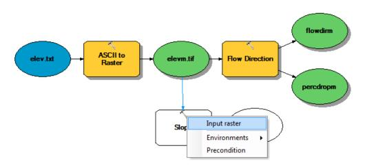
Add the **Spatial Analyst**  $\rightarrow$  **Surface**  $\rightarrow$  **Aspect** tool to your model connecting it to elevm.tif as an input in a similar way. Double click on the Slope and aspect tool outputs and specify file names for the outputs.
