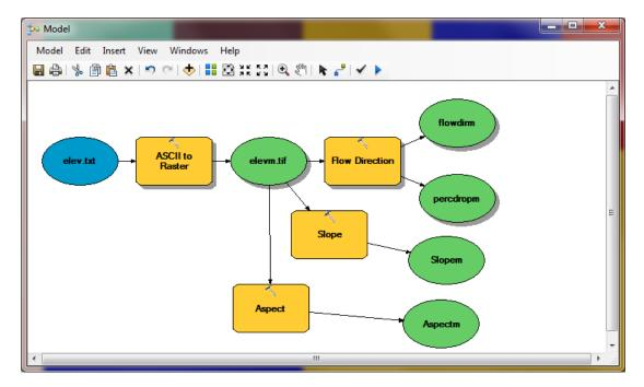
You can click run and do all the processing required to import the data, compute Slope, Aspect, Flow Direction and Hydrologic Slope at the click of a single button. Pretty slick!
