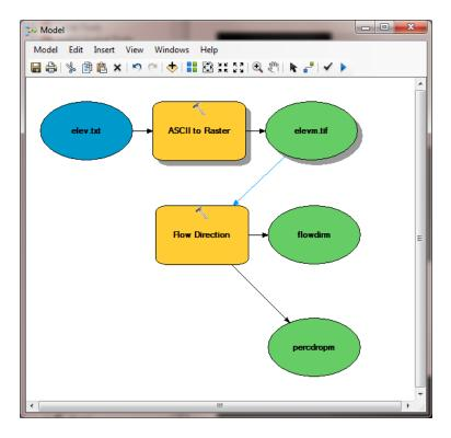
The orange boxes briefly flash red as each step is executed. The Model progress box opens and the progress bar indicates when the model completes. You can then add the outputs to the map and examine the results.
