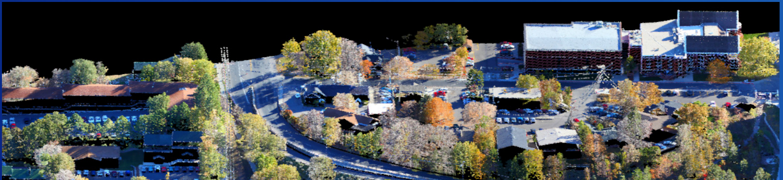
Helicopter swath through Utah State University from 200 m using Riegl Q560 lidar system
