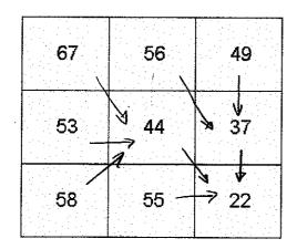
(1) Determine the flow direction in each cell and label it using the ESRI 8-direction pour point method (1, 2, 4, 8, 16, 32, 64, 128)
