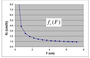
4. Ponding (saturation at the surface) first occurs when  $f_c=W$  (water input rate or rainfall rate) This idea lets you solve for the depth of water that has to infiltrate before ponding occurs,  $F_p$ , and the time to ponding  $t_p$  for a particular input rate W.
