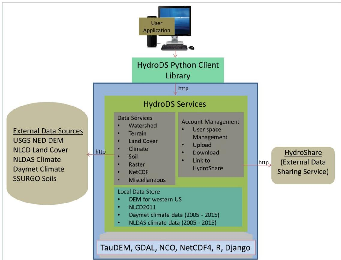
Figure 3. High-level architecture of HydroDS. HydroDS comprises HydroDS Services and HydroDS Python Client Library.
