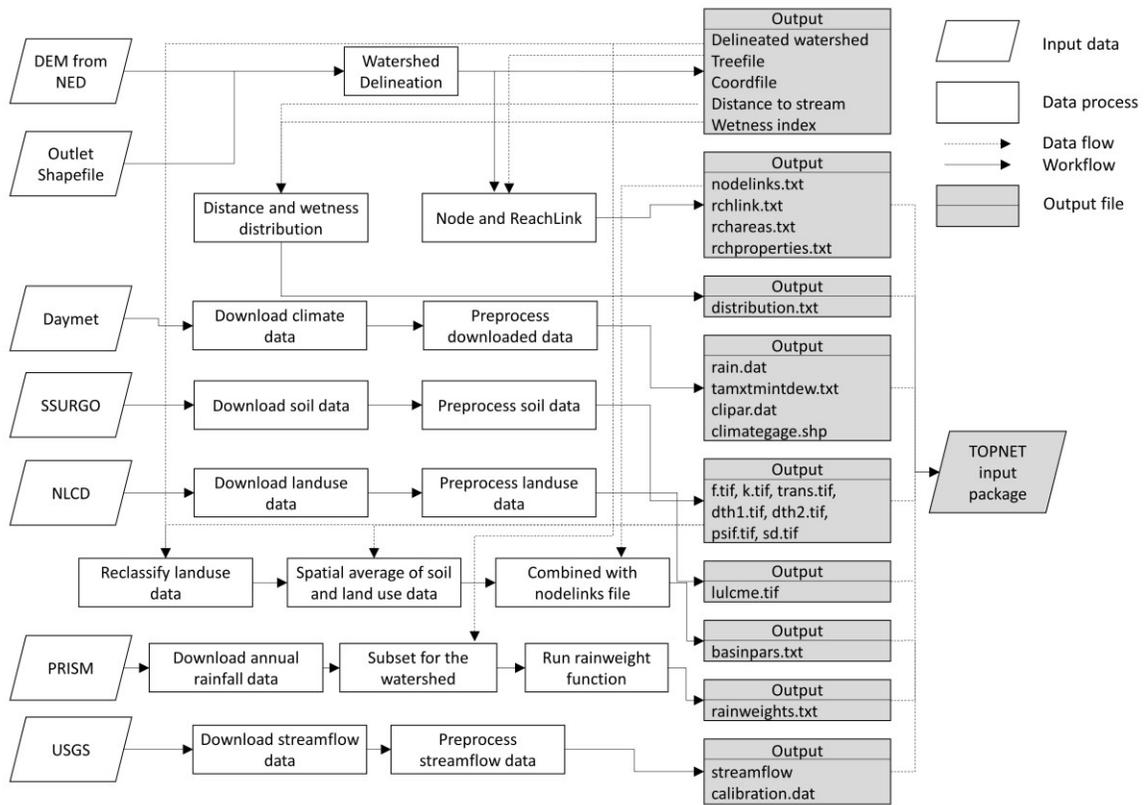
Figure 2. Input data pre-processing steps for TOPNET model
