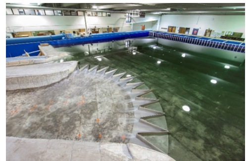
Figure 1.(a) 1:45 scale model of Lake Isabella labyrinth spillway (Photo credit: UWRL, Blake Tullis)
