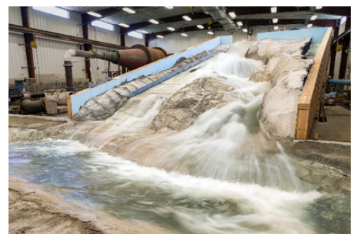
Figure 1.(b) 1:50 scale model of the damaged Oroville Dam spillway (Photo credit: USU, Matt Jensen)
