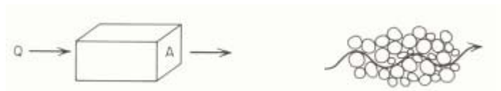
Figure 24. Macroscopic and microscopic concepts of porous medium flow (Freeze/Cherry, Groundwater , © 1979. Electronically reproduced by permission of Pearson Education, Inc., Upper Saddle River, New Jersey).
