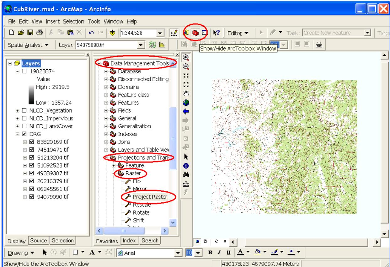
In the Project Raster dialog that opens specify the input raster as the National Elevation Dataset DEM that was unzipped from the download. Name the output raster something convenient. Here I used "cubdem". Click on the button next to Output coordinate system to open the Spatial Reference Properties dialog.
