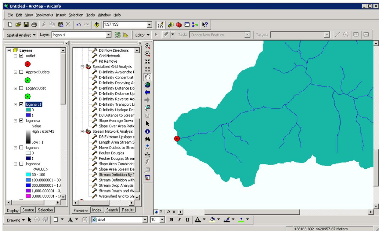
13. This network is still only represented as a grid. To convert this into vector elements represented using a shapefile, the **Stream Reach and Watershed** function is used.
