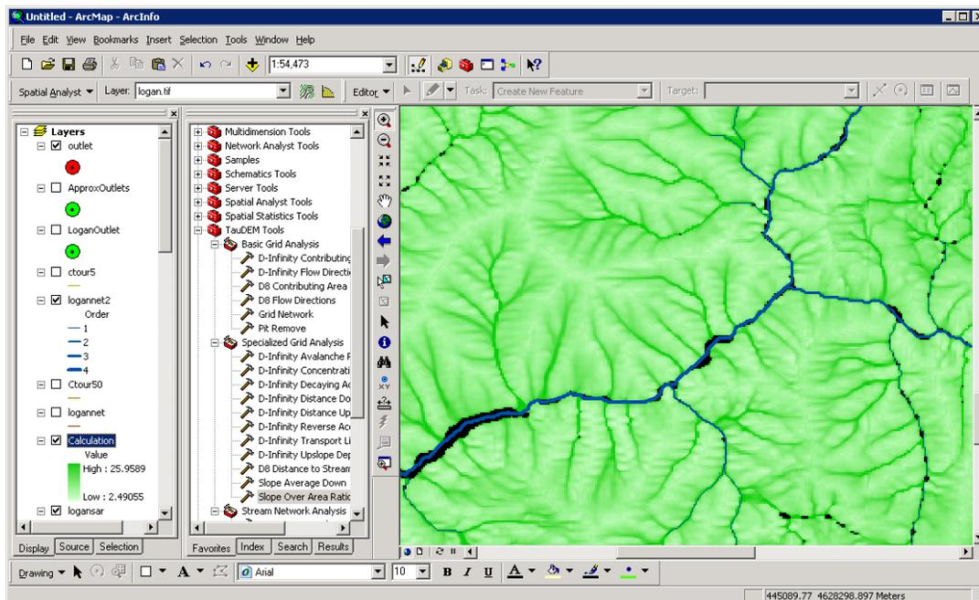
18. The **D-Infinity Distance Down** function computes the distance to streams (or any designated target grid) a number of different ways
