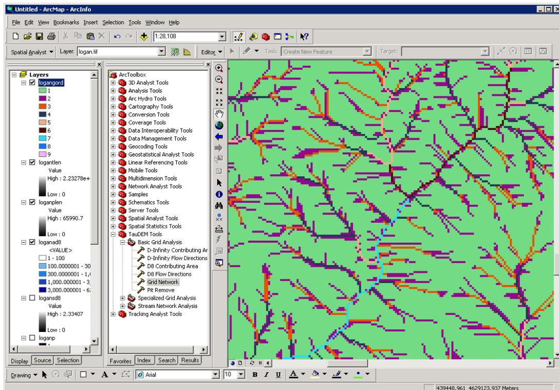
The functions above used the D8 flow model that represents flow from each grid cell to one neighbor. TauDEM also uses the  $D_{\infty}$  (D-Infinity) flow model that calculates the steepest outwards flow direction using triangular facets centered on each grid cell and apportions flow between neighboring grid cells based on flow direction angles.
