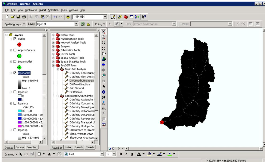
12. The next step is to use the **Stream Definition By Threshold** function to define streams using a specified contributing area threshold. Here a threshold of 2000 grid cells is arbitrarily chosen
