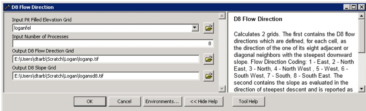
The resulting D8 flow direction grid (grid has suffix p) is illustrated. This is an encoding of the direction of steepest descent from each grid cell using the numbers 1 to 8 per the embedded help above. This is the simplest model of the direction water would flow over the terrain.
