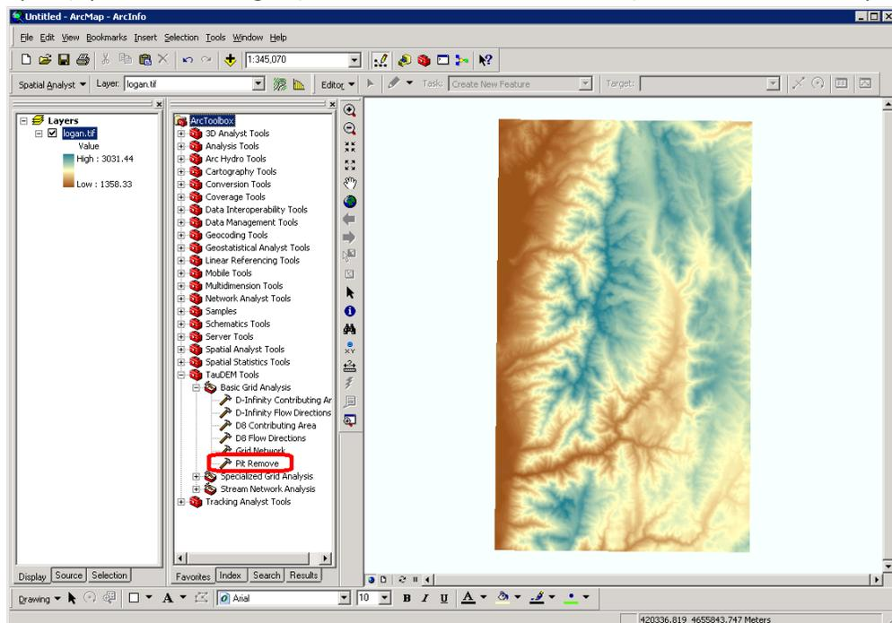
Select **logan.tif** for the Input Elevation Grid. Note that the Output Pit Removed Elevation Grid name is automatically filled with loganfel.tif following the file naming convention. Select the Input Number of Processes (I used 8 for a dual quad core PC).
