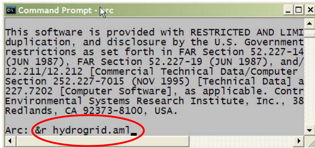
Figure 2.5. Command to run hydrogrid.aml.
