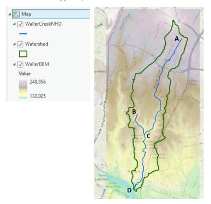
The file austin.zip provided for problem 3 includes a 10 m digital elevation model (DEM) for this area obtained from the National Map (WallerDEM) and the NHD streams within the Waller Creek Watershed, both projected into UTM coordinates.
