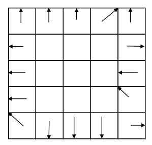
c) Determine the **flow accumulation grid** corresponding to the D8 flow directions. Label each cell on the grid below with the number of upstream cells draining **into it** (ESRI convention). What is the maximum flow accumulation value in this internal grid (the 9 cells with no arrows in them)?
