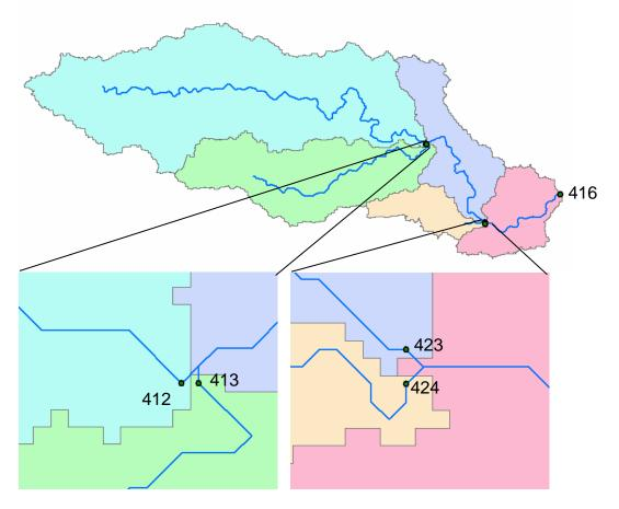
The drainage points have each been labeled with their HydroID. Following are the corresponding attribute tables. The units are km for length and  $km^2$  for area.
