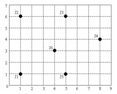
5. A set of 6 elevation points has been obtained by aerial photogrammetry, as shown in the table and figure below. Construct a Delauney triangulation of these points. Use this triangulation to draw the 50 m, 40 m and 30 m contours. Please make a neat solution for the contours but don't spend a huge amount of time trying to make them highly precise.
