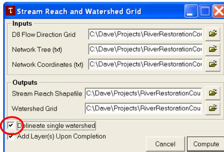
The Watershed Grid that is output is a single watershed for the entire Cub River upstream of the outlet point. Use the Watershed Grid to Shapefile function to create a Shapefile of this watershed.
